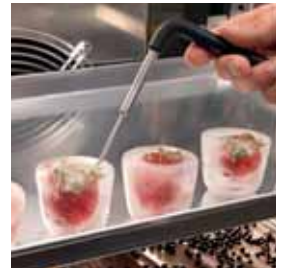
Sonda rilevamento temperatura Probe to survey the core temperature of the product
