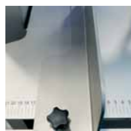
Scala graduata sul piano di lavoro Worktop with graduated scale
