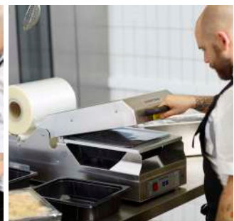
4. The machine opens automatically once the tray is sealed (except manual machines DF10/15).
